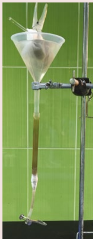
The Baermann technique is based on the active migration of the larvae (L1). Faeces are suspended in water: the larvae move into the water and sink to the bottom, where they can be collected for identification.
